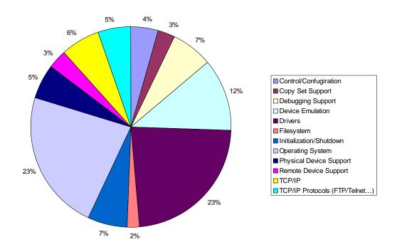
As the graph shows, the basic operating kernel accounts for about 24% of the total code, kernel support (initialization, shutdown, debugging commands, configuration) is about 16%, device drivers and device control about 30%, TCP/IP and TCP/IP utilities 12%, and the application code 18%.
